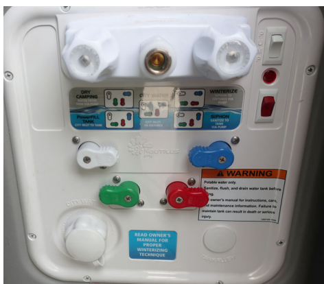
Water Center Panel in “Winterize” configuration (Panel located behind passenger rear door). -Typical view
