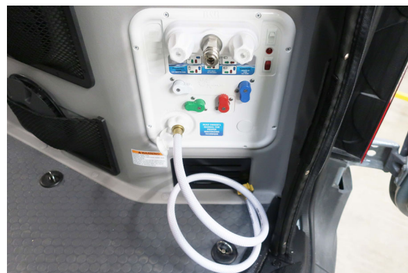
Attach a siphon tube then place it in the chlorine solution container and turn the pump on to begin siphoning contents. (typical view)
